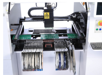
Internal conveyor system
